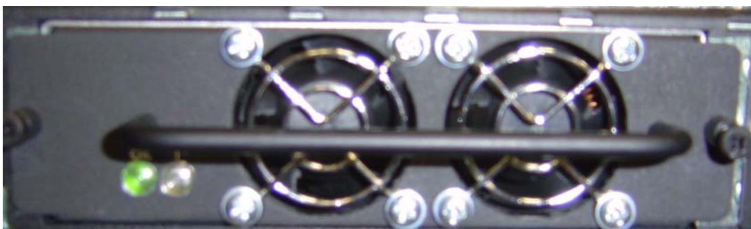
Figure 5-2: Power Supply LEDs
